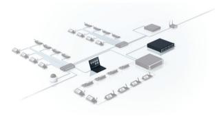
The DICENTIS System Software is used as a platform for controlling the entire DICENTIS Conference System. Basic functions are included; additional functions can be added depending on the required functionality.
